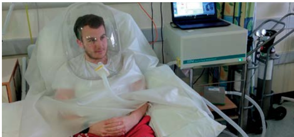
One of our volunteers wearing the indirect calorimetry ‘hood’, which measures the oxygen and carbon dioxide in the exhaled breath of the wearer.
